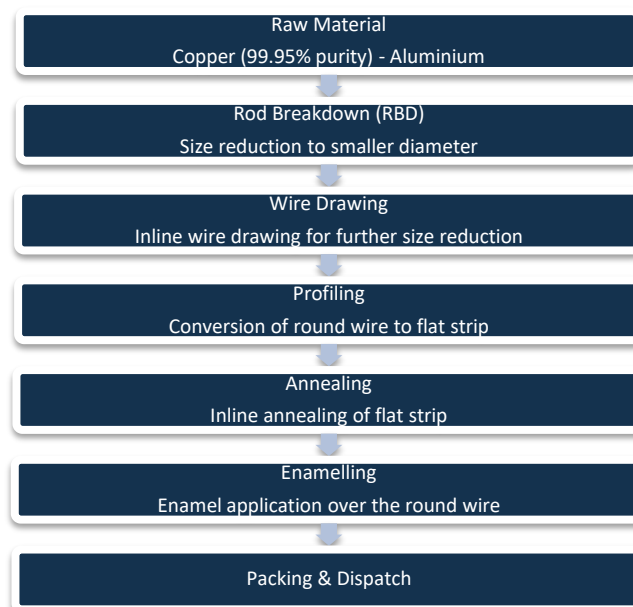
Chart 17: Process flow of manufacturing of Enamelled Copper/Aluminium Magnet Winding Wires
