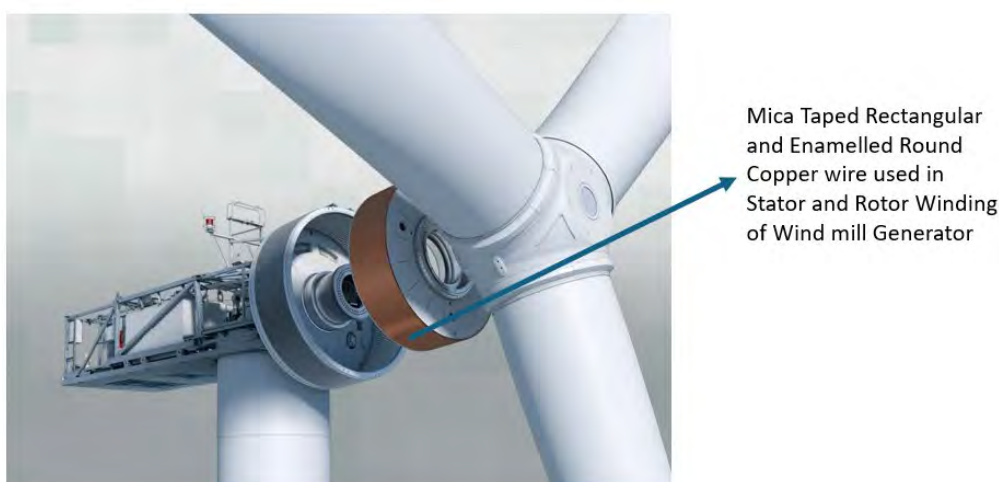
Figure 2: Use of Winding Wires in Turbine Generator
